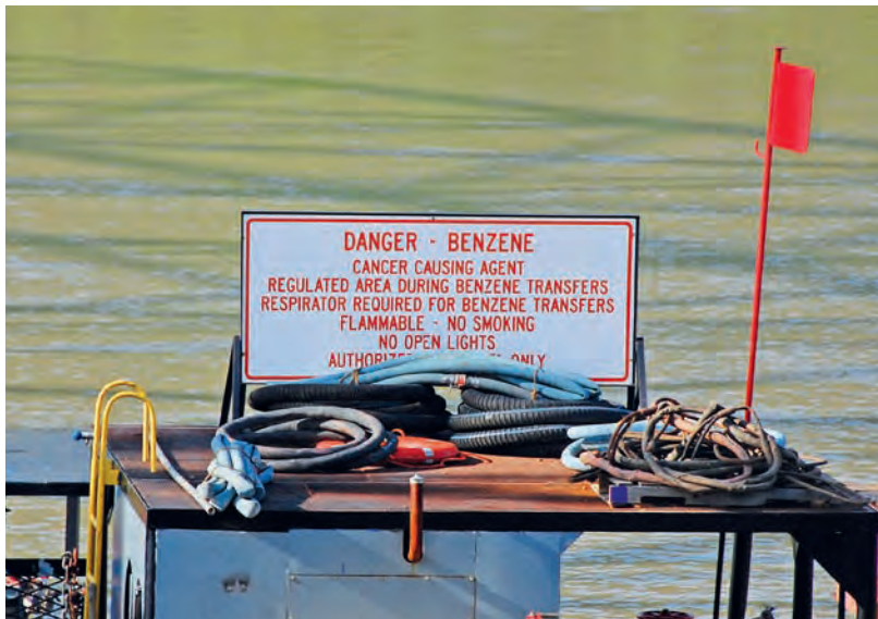
Fig. 2.10.1. If there is a requirement to continue using and distributing a chemical known to be carcinogenic to humans, specifically in an occupational context, a range of preventive measures may be implemented, in this case illustrated by warning signs concerning benzene in the USA.
