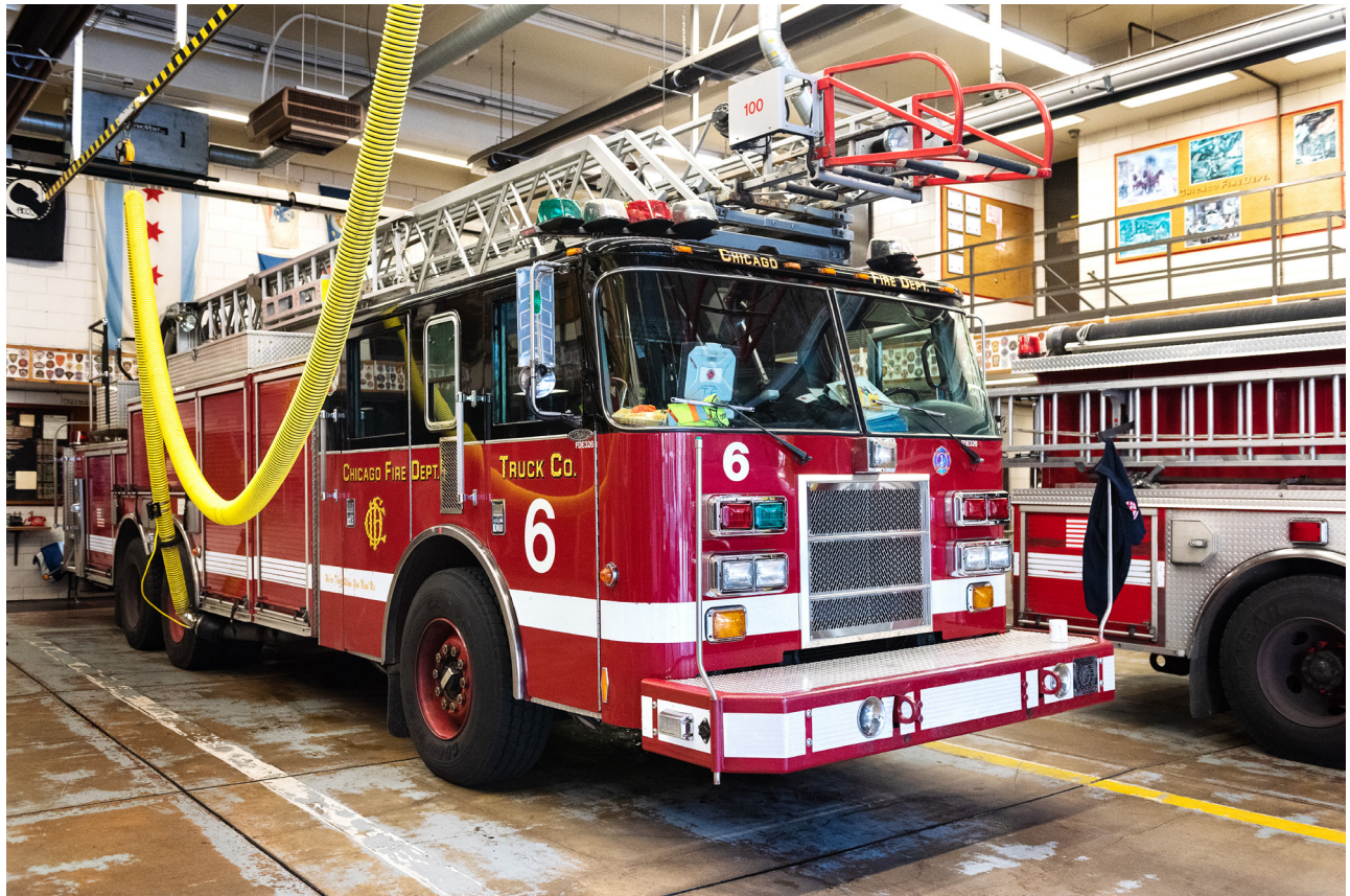
Fig. 1.7 Fire station in Chicago, USA, with diesel-exhaust capture system attached to a fire truck
