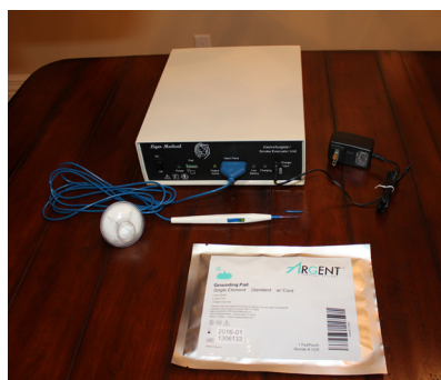
Fig. 5.5. A portable, battery-driven electro-surgical unit incorporating a suction unit. Ports for the electro-surgical pencil and the ground plate are displayed. A simple electrical battery charger access point and the on/off switch complete the display at the front. The suction port site is at the rear of the unit.
