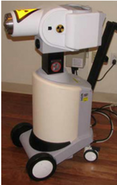
Fig. 15.3. High-dose-rate remote afterloading brachytherapy machine.
