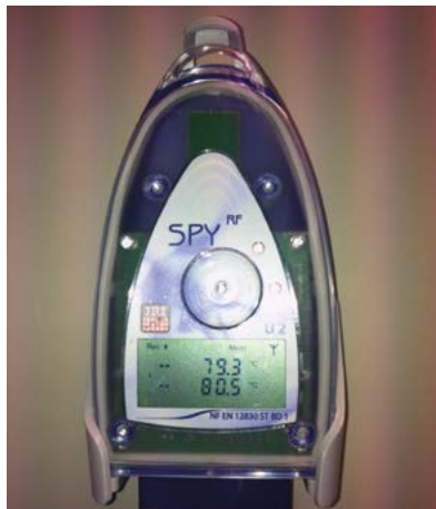
Fig. 9. Temperature monitoring system.
