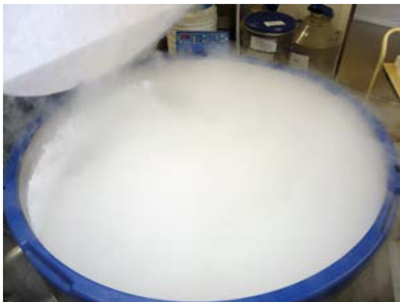
Fig. 6. Tank for storage in vapour-phase liquid nitrogen.
