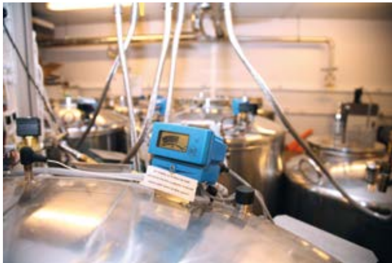
Fig. 13. A tank fitted with a monitoring device, which shows the level of liquid nitrogen inside the tank.
