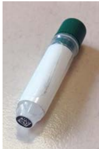
Fig. 26. Pre-labelled tube with two-dimensional barcode.
